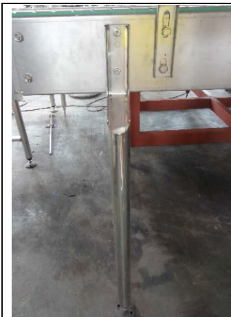
The conveyor and feet are made in one piece.
